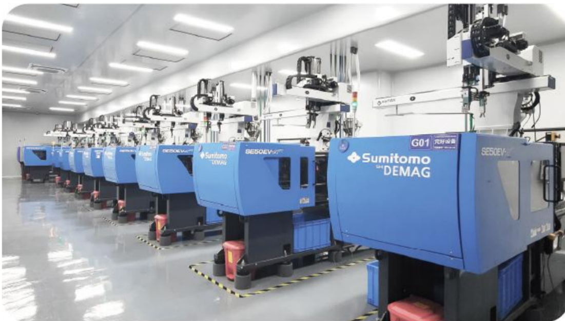
▲ Cleanroom Molding Zone(Class 100,000) SE50-100 series
